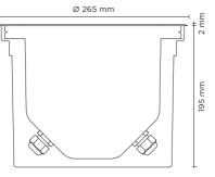
HOLE FOR RECESSING Ø 257 mm
