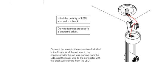
Fix the rest of the fixture by screwing it onto the installation part
