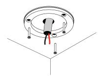
Fix the installation part with the 3 screws
