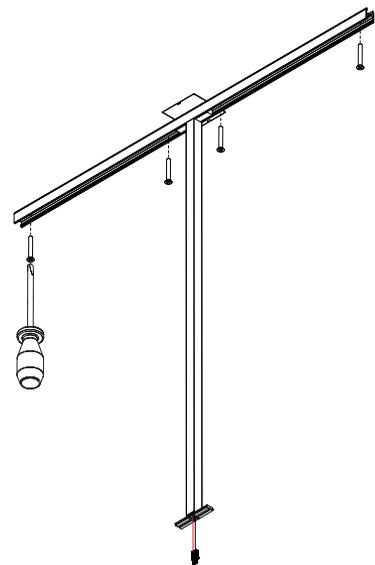
fixate the ceiling profile with four screws
