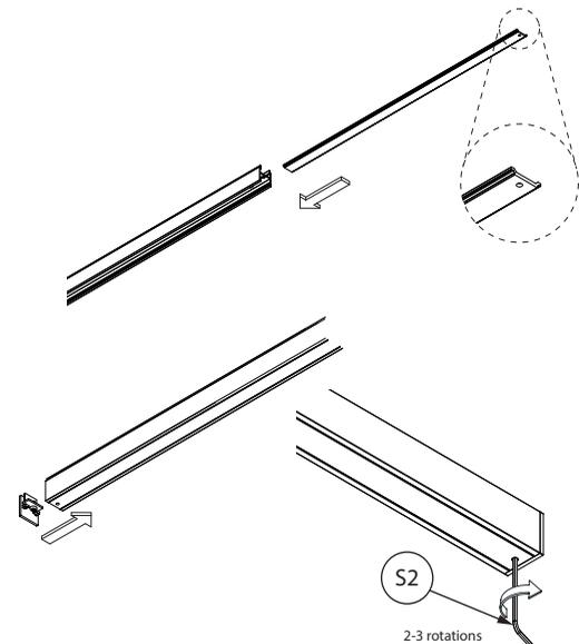
slide the covers back into place (make sure the hole is on the outside) then put the end-caps back and fixate them with the hexagon key
