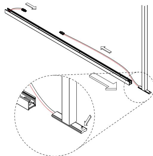
slide the LED-element on the vertical from the correct side! make sure the connectors are pointed towards each other and that the set screw is positioned on the other side!
