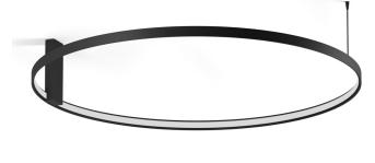
Ceiling or wall lighting fixture for interiors, with direct and indirect light emission. Pickled sheet metal ceiling or wall bracket in polyacrylic paint. Pickled sheet metal wall plate in polyacrylic paint. Bended extruded aluminium structure in white, black, bronze, mat brass or titanium polyacrylic paint.
