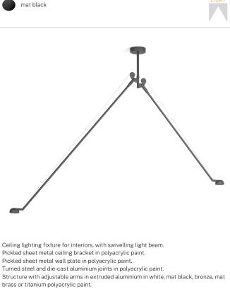
Steel wire rope slings. Die-cast aluminium heads rotating on two axes in polyacrylic paint. Modelled polycarbonate diffusers with opaline finish and serigraphy.
