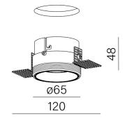
Tolerance for dimensions  $\pm 1$ mm
