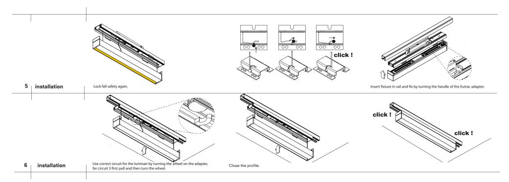
To uninstall the fixture follow the steps from line 2 on sheet 1, turn the circuit wheel to 0 (line 6) unlock the eutrac adapter (line 5).
