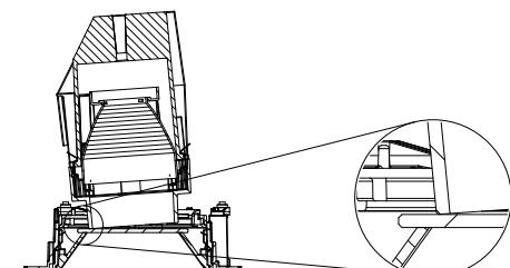
mod 80/120:led module can not rotate when the IP44 louvre is installed
