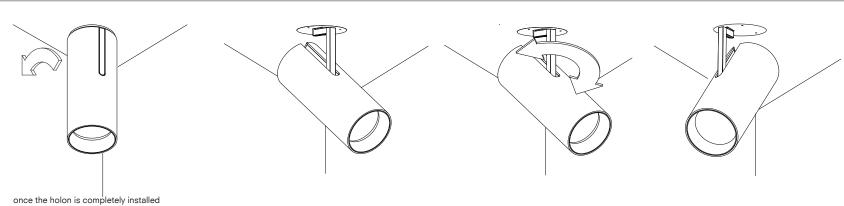
it can be inclined in any angle up to 90° by pullin the tube
