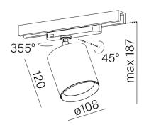
Tolerance for dimensions ± 1mm
