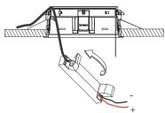
install the correct gear with strain relief on the hollow ceiling
