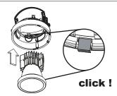
insert the reflector-LED assembly in the Aplis the border of the reflector has to snap on the springs
