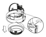
Bend the springs to remove the filterholder.
