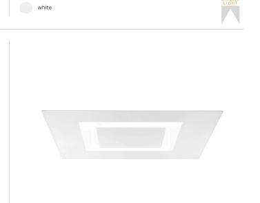
Lighting fixture for ceiling built-in installation for interiors, with direct light emission. Built-in bearing structure for modular false ceilings, in aluminium in polyacrylic paint. Pickled sheet metal closing frames in white polyacrylic paint. Modelled polycarbonate diffuser with opaline finish. Equipped with inspection flap to access the terminal block.
