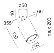
Tolerance for dimensions ± 1mm
