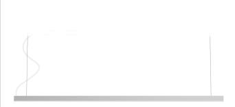
Suspension lighting fixture for interiors, with direct light emission. Extruded aluminium structure in RAL 9003 white powder paint. Extruded aluminium reflector in powder paint. Extruded polycarbonate diffuser with opaline finish. Aluminium end caps in polyacrylic paint. Suspension kit with griplocks and 2m (78,7") long steel cables. 2,2m (86,6") long power cable in transparent PVC. Power canopy with pickled sheet metal ceiling bracket and covering in white polyacrylic paint.
