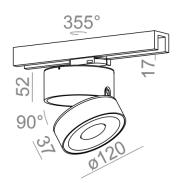
Tolerance for dimensions ± 1mm
