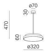
Tolerance for dimensions  $\pm 1$ mm
