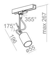
Tolerance for dimensions ± 1mm
