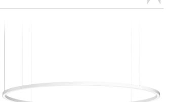
Suspension lighting fixture for interiors, with direct light emission. Bended extruded aluminium structure in white, black or mat brass polyacrylic paint. Extruded polycarbonate diffuser with opaline finish. Suspension kit with griplocks and 5m (196,9") long steel cables. 5m (196,9") long power cable in transparent PVC. Power canopy with pickled sheet metal ceiling bracket and covering in white polyacrylic paint.
