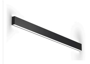
Wall lighting fixture for interiors, with direct and indirect light emission. Extruded aluminium structure in RAL 9003 white or black powder paint. Extruded polycarbonate diffusers with opaline finish. Pickled sheet metal end caps in polyacrylic paint.
