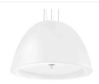
Suspension lighting fixture for interiors, with direct and indirect light emission. Turned pickled sheet metal structure in metallized grey polyacrylic paint. Extruded aluminium heat sink. Moulded polyethylene lampshade in white colour. Diffuser in modelled frosted glass. 2m (78,7") long steel suspension cables. 2,2m (86,6") long power cable in transparent PVC. Power canopy with galvanized sheet metal ceiling bracket and pickled sheet metal covering in metallized grey polyacrylic paint.
