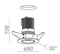
Tolerance for dimensions ± 1mm
