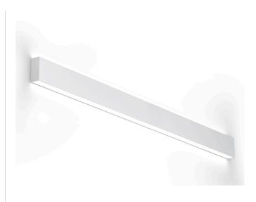
Wall lighting fixture for interiors, with direct and indirect light emission. Extruded aluminium structure in RAL 9003 white or black powder paint. Extruded polycarbonate diffusers with opaline finish. Pickled sheet metal end caps in polyacrylic paint.
