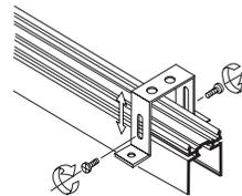
the height of bracket can be adjusted to the thickness of the ceiling to ensure a flush mount
