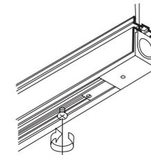
first turn all screws clockwise 90° until track site flush in the support profile, starting from the middle and working outwards
