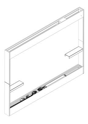
electric part: connect the black 5P female connector to the black 5P male connector coming from the gear.
