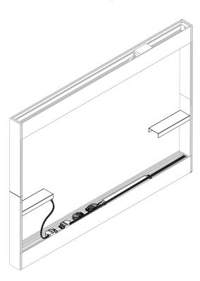
audio part: lead the white 4P female connector with the cable underneath the audio speakers and connect it to the 4P male connector coming from one of the speakers. Make sure the cable is pulled tight, so there's no cable interfering with the cover.
