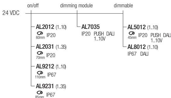
**Note:** dimming module AL7035 to be used in combination with a 24VDC power supply
