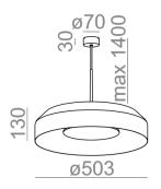
Tolerance for dimensions ± 1mm
