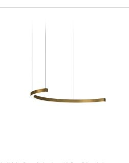
Suspension lighting fixture for interiors, with direct light emission. Bended extruded aluminium structure in white, black or mat brass polyacrylic paint. Extruded polycarbonate diffuser with opaline finish. Galvanized sheet metal end caps in polyacrylic paint. Suspension kit with griplocks and 2m (78,7") long steel cables. 2,2m (86,6") long power cable in transparent PVC. Power canopy with pickled sheet metal ceiling bracket and covering in white polyacrylic paint.
