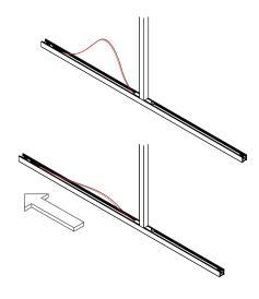
slide the LED asymmetrical. Make sure the vertical profile slides away from the connectors
