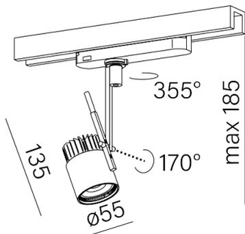
Tolerance for dimensions ± 1mm
