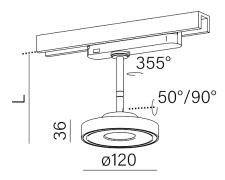
Tolerance for dimensions ± 1mm
