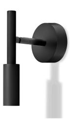
Ceiling or wall lighting fixture for interiors, with swivelling light beam. Galvanized sheet metal ceiling or wall bracket. Die-cast aluminium wall plate in white, champagne, mat black, bronze or titanium polyacrylic paint. Turned brass joints in polyacrylic paint. Turned aluminium structure in polyacrylic paint. Turned aluminium head rotating on two axes in polyacrylic paint.
