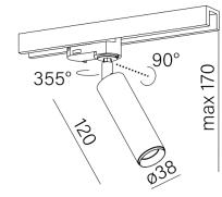
Tolerance for dimensions ± 1mm
