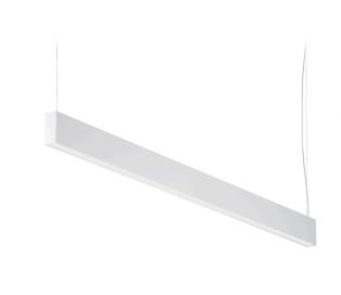
Suspension lighting fixture for interiors, with direct and indirect light emission. Extruded aluminium structure in RAL 9003 white or black powder paint. Extruded polycarbonate diffusers with opaline finish or micro-prismatic. Pickled sheet metal end caps in polyacrylic paint. Suspension kit with griplocks and 2m (78,7") long steel cables. 2,2m (86,6") long power cable in transparent PVC. Power canopy with galvanized sheet metal ceiling bracket and pickled sheet metal
