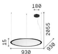
Net weight 5.4 kg Insulation class Ī **Protection index** IP20 Compliance CE **Operating temperature** 0° ~ +40 °C
