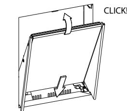
insert the reflector, underside first.
