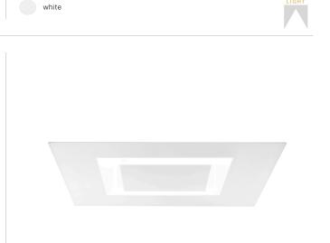
Lighting fixture for ceiling built-in installation for interiors, with direct light emission. Built-in bearing structure for modular false ceilings, in aluminium in polyacrylic paint. Pickled sheet metal closing frames in white polyacrylic paint. Modelled polycarbonate diffuser with opaline finish. Equipped with inspection flap to access the terminal block.
