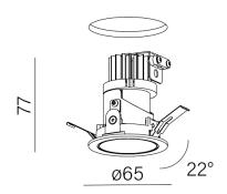
Tolerance for dimensions ± 1mm
