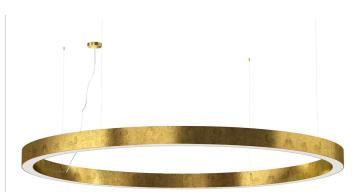
Pickled sheet metal structure in polyacrylic paint. Aluminium dissipation plates. Aluminium and pickled sheet metal covers in white or black polyacrylic paint, or with gold leaf coating. Diffusers in modelled polycarbonate with opaline finish. Suspension kit with griplocks and 5m (196,9") long steel cables. 5m (196,9") long power cable in transparent PVC.
