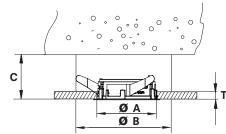
\*In case of standard driver (KR772024/ KR772022/KR772122) which needs to be pushed through the plasterkit In case of driver placed at distance (doesn't need to be pushed through the plasterkit) Cmin = 60 In case of a different driver, the installation dept Cmin = length of driver + 30 mm
