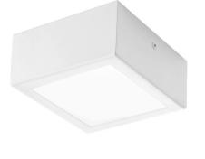
Ceiling or wall lighting fixture for indoor or outdoor spaces, with direct light emission. Ceiling/wall plate in die-cast aluminium in metallized grey polyacrylic paint. AISI 316 stainless steel structure in white or metallized brown polyacrylic paint. EPDM rubber gasket. Aluminium dissipation plate. Flat frosted glass diffuser. Rubber cable grommet. Stainless steel screws.
