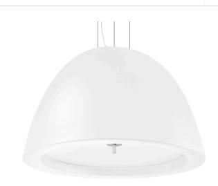
Suspension lighting fixture for interiors, with direct and indirect light emission. Turned pickled sheet metal structure in metallized grey polyacrylic paint. Moulded polyethylene lampshade in white colour. Diffuser in modelled frosted glass. 2m (78,7") long steel suspension cables. 2,2m (86,6") long power cable in transparent PVC. Power canopy with galvanized sheet metal ceiling bracket and pickled sheet metal
