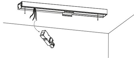
Connect female connector with strain relief to powersupply and dali dim.
