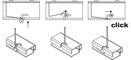
Add cable to fall safety at both ends. When profile is >2,5m one extra fall safety in the middle.
