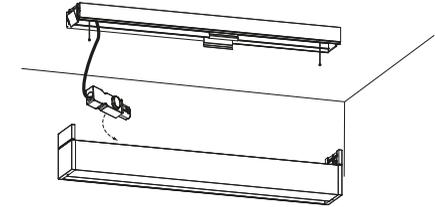
Make correct connection with male connector in the luminaire.
