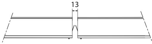
In case of several pieces install the profiles with 13mm distance between the upper extrusions.
