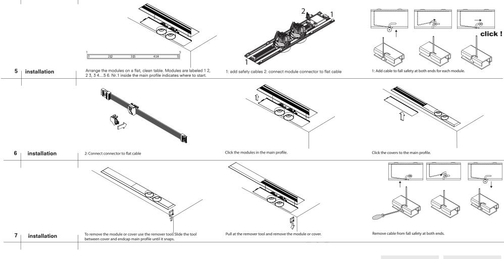
When the fall safety is unlocked, support the profile to avoid falling.
