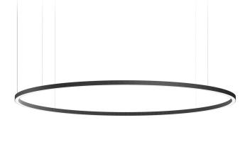
Suspension lighting fixture for interiors, with direct light emission. Bended extruded aluminium structure in white, black or mat brass polyacrylic paint. Extruded polycarbonate diffuser with opaline finish. Suspension kit with griplocks and 5m (196,9") long steel cables. 5m (196,9") long power cable in transparent PVC. Power canopy with pickled sheet metal ceiling bracket and covering in white polyacrylic paint.
