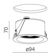
Tolerance for dimensions ± 1mm
