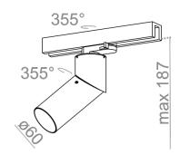
Tolerance for dimensions  $\pm 1$ mm
