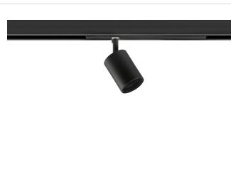
Lighting fixture for electrified track for interiors, with swivelling light beam. Die-cast aluminium joint with powder paint. Die-cast aluminium structure rotating on two axes in white or black powder paint. Acrylic moulded lens. Anti-glare snoot in black thermoplastic material.
