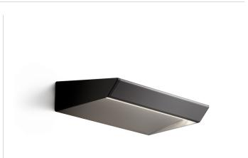
Wall lighting fixture for interiors, with direct and indirect light emission. Pickled sheet metal wall bracket in polyacrylic paint. Extruded aluminium structure in white, black, bronze, mat brass or titanium polyacrylic paint. Extruded acrylic diffusers with opaline finish.
