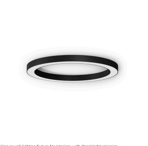
Ceiling or wall lighting fixture for interiors, with direct light emission. Pickled sheet metal ceiling/wall bracket in polyacrylic paint. Pickled sheet metal structure in polyacrylic paint. Aluminium dissipation plates. Pickled sheet metal covers in white, black or bronze polyacrylic paint, or with gold leaf coating.
