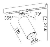
Tolerance for dimensions ± 1mm
